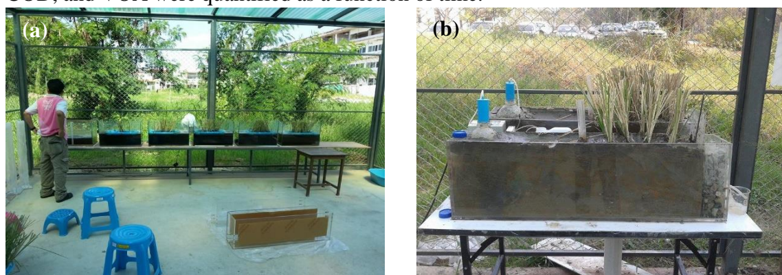
Figure 5. (a) Laboratory-scale vetiver grass in a floating platform and (b) Laboratory-scale PRVRB.
